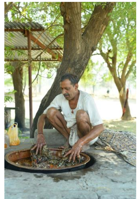
Figure 7 Printer Purushottam Chhipa dyeing cloth in a submerged copper dye pot. Photo courtesy of Wabisabi and Anokhi Archives.
