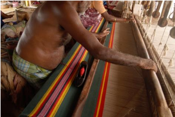
The chukka-pidittal process forms a zig-zag to allow the yarn to pass over and under the warp, creating a ribbed effect.
