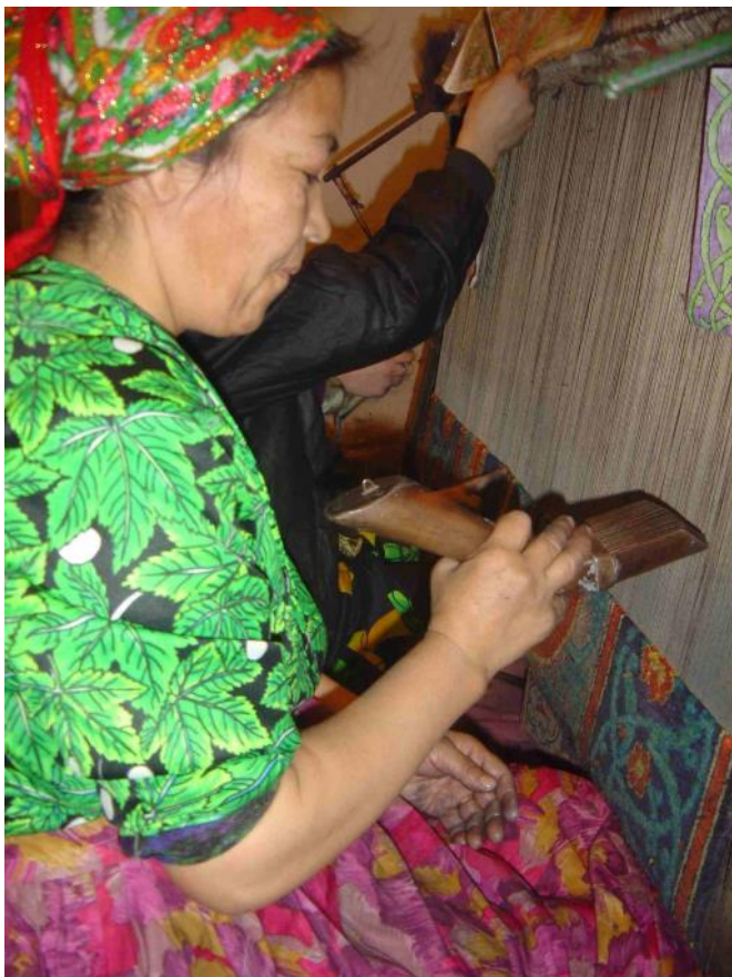
Beating down the knots and the weft with a weaver's comb. 2004. Photo: Chris Alexander.
